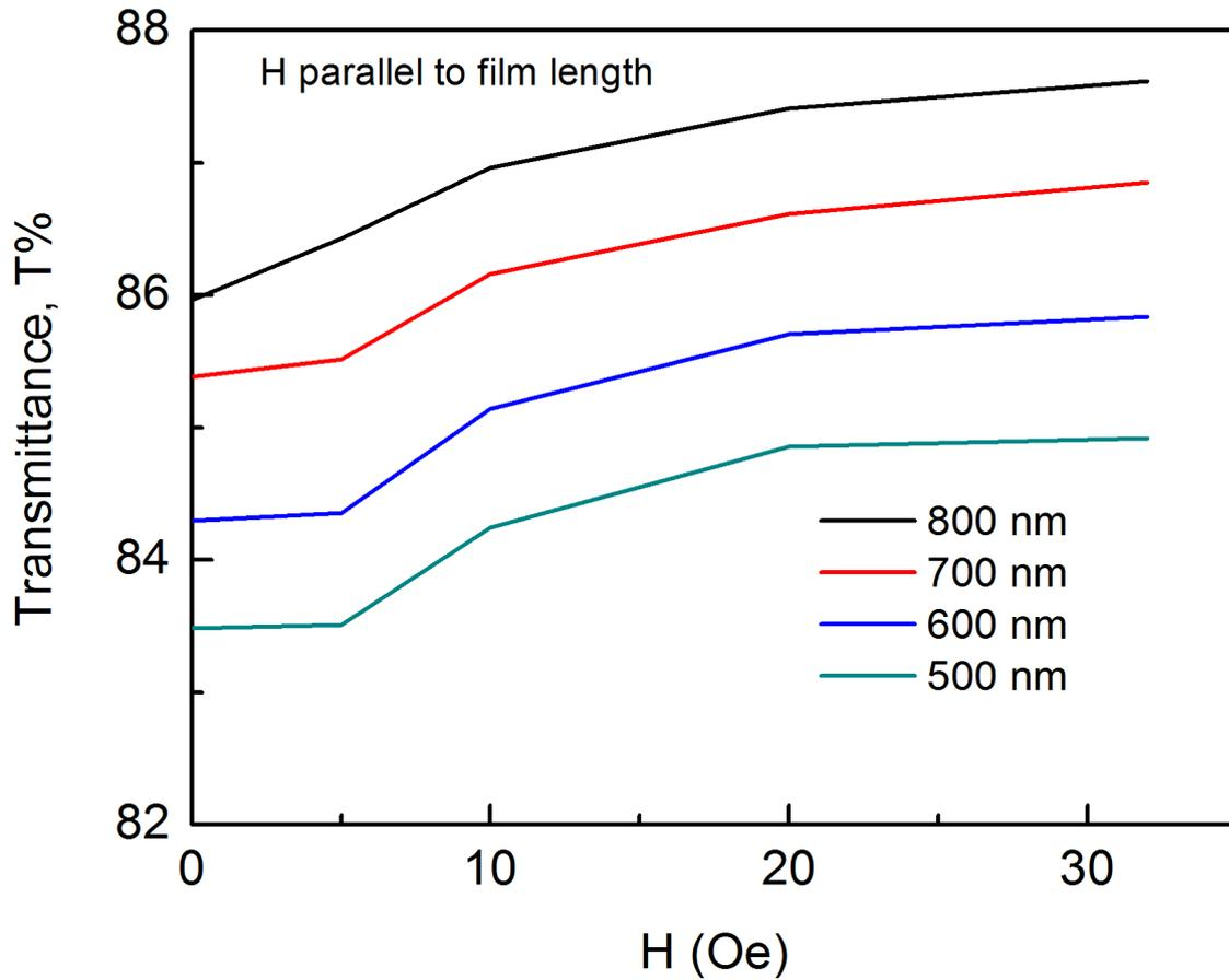
Figure 4. The variation of the transmittance as a function of magnetic field with fixed wavelengths for  $\text{Fe}_3\text{O}_4$  particles with  $10 \mu\text{m}$  film in parallel magnetic field.
