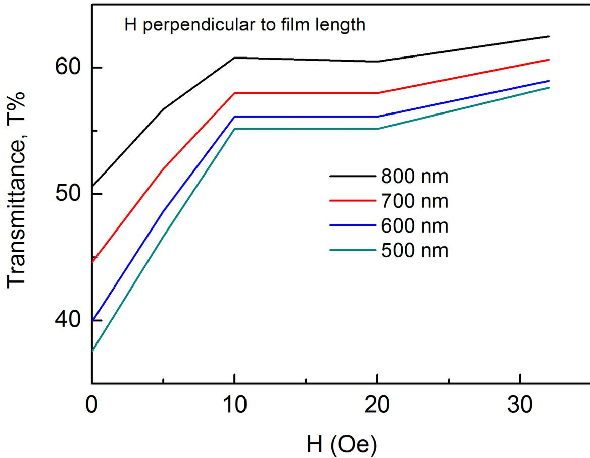
**Figure 2. The variation of the transmittance as a function of magnetic field with fixed wavelengths for Fe<sub>3</sub>O<sub>4</sub> particles with 10 μm film in perpendicular magnetic field.**
