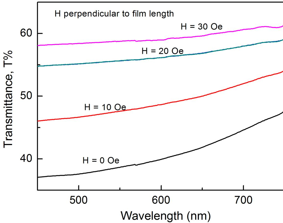
**Figure 1.** The variation of the transmittance as a function of wavelength with a various applied magnetic fields for Fe<sub>3</sub>O<sub>4</sub> particles with 10 μm film in perpendicular magnetic field.
