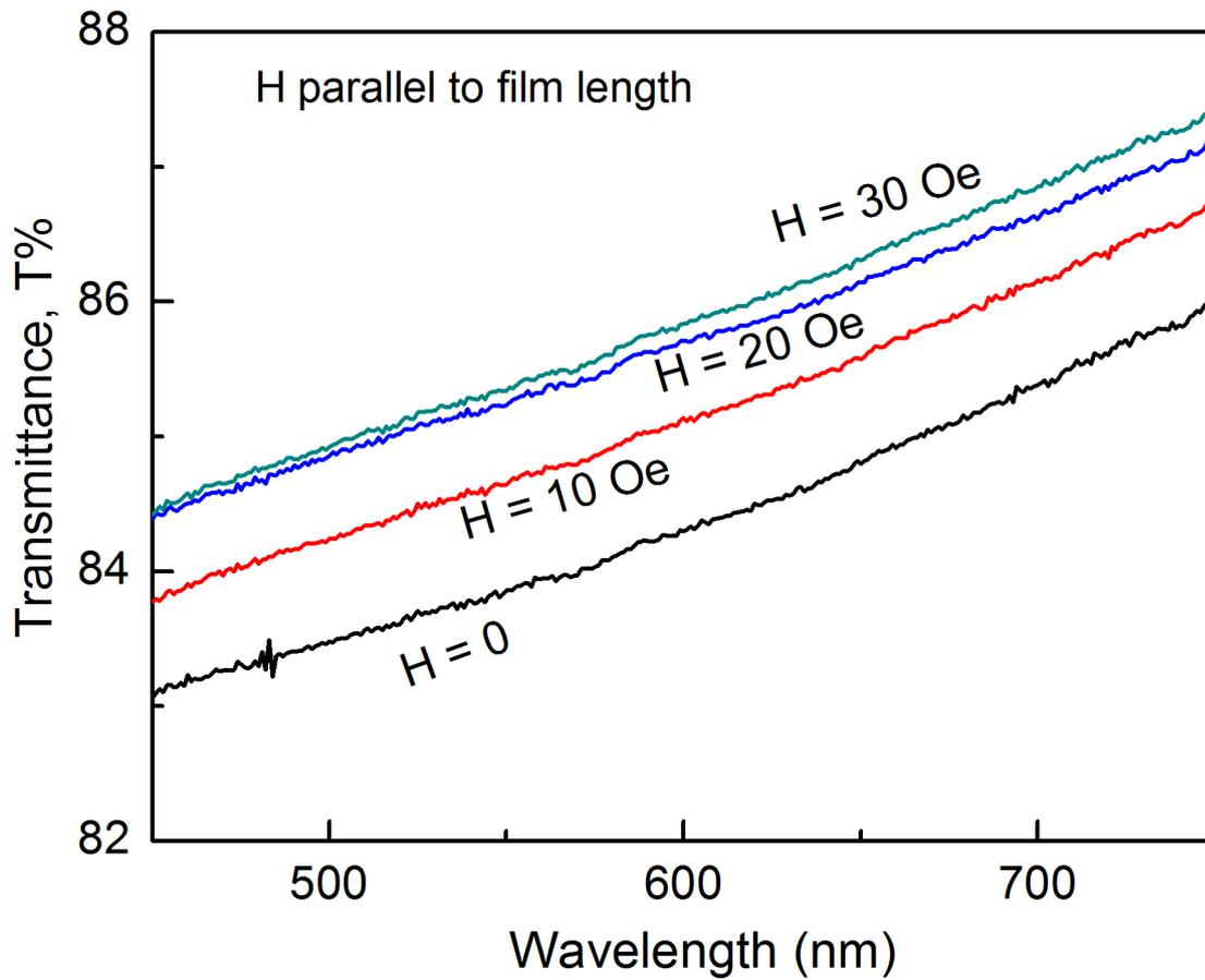
**Figure 3.** The variation of the transmittance as a function of wavelength with a various applied magnetic fields for  $\text{Fe}_3\text{O}_4$  particles with  $10 \mu\text{m}$  film in parallel magnetic field.
