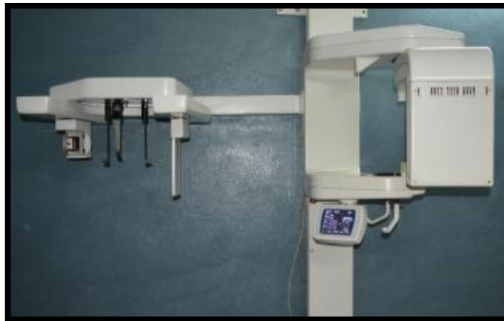
Figure 6: Digital cephalostat with functional head positioners
