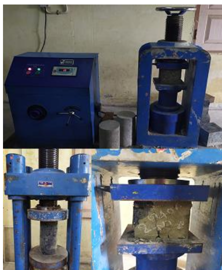
Fig. 7 Compression Testing on Concrete Specimens
