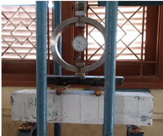
Fig. 9 Closer view of Flexural Testing of Concrete
