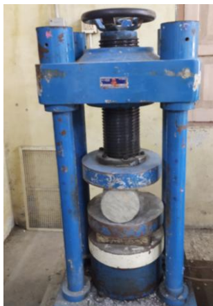
Fig. 10 Tension Testing on Concrete
