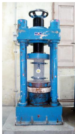
Fig. 11 Modulus of Elasticity Test on Concrete
