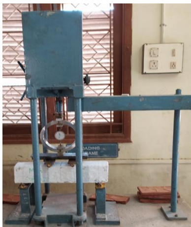
Fig. 8 Flexural Testing of Concrete
