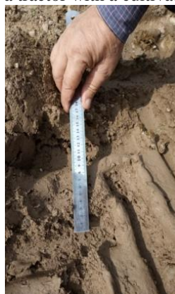
Figure 10- Spot measurements of tractor pneumatic tires under various loads: a) tractor without an aggregate; b) a tractor with a cultivating unit; c) tractor with fertilizer cultivator.
