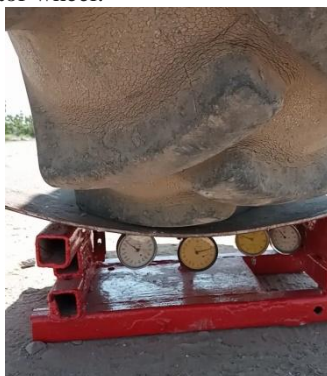
Figure 2- The indicator of the clock model Ich-150 (tire pressure 0.10 MPa) of the driving wheel 13.6 R38 ЯR-318 for determining the deformation properties: 1-fixed frame (installation frame); 2-locking bolt; 3-tensile resistant; 4-movable support (plate).
