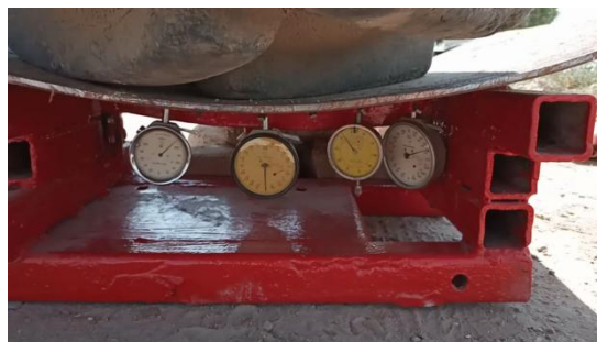
Figure 2- The indicator of the clock model Ich-150 (tire pressure 0.10 MPa) of the driving wheel 13.6 R38 ЯR-318 for determining the deformation properties: 1-fixed frame (installation frame); 2-locking bolt; 3-tensile resistant; 4-movable support (plate).
