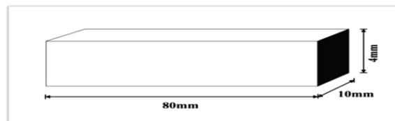
Figure (7) dimensions and measurement of the impact test samples
