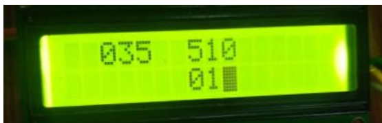
Figure 19: LCD output of the person IN/OUT count, temperature and humidity level of monitoring system
