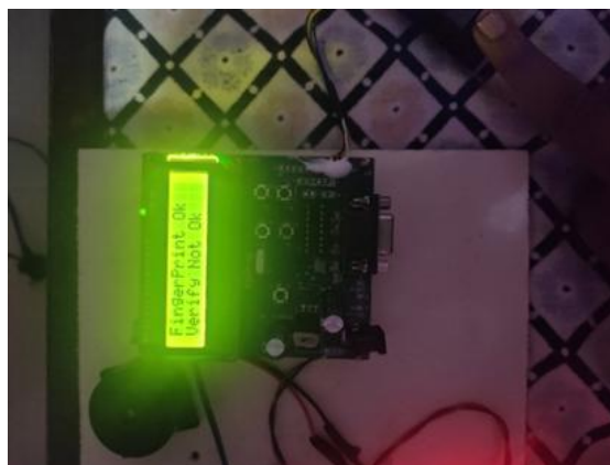
Fig.26. Fingerprint is not matched and the not ok command is displayed
