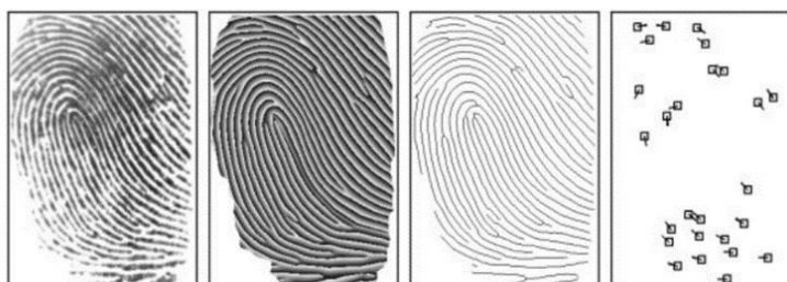
Fig.5. Minutiae Algorithm Working Principle
