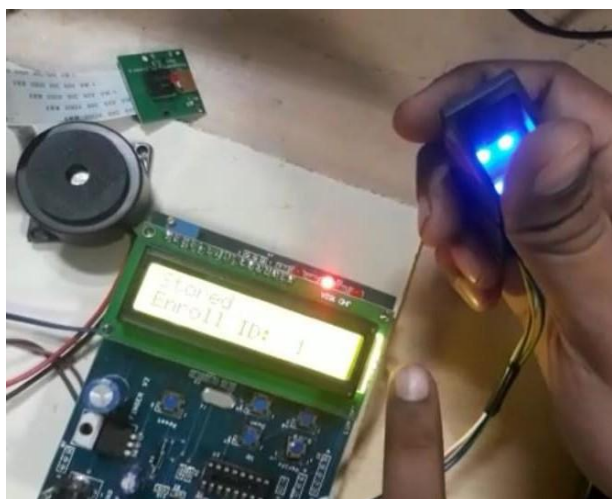
Fig.3. Fingerprint is stored in Database
