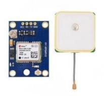
The NEO-6MV2 is an GPS (Global Positioning System) module and is employed for navigation. The module simply checks its location on earth and provides output data that is line of longitude and latitude of its position. It is from a family of complete GPS receivers that includes the high performance u-blox 6 positioning engine.
