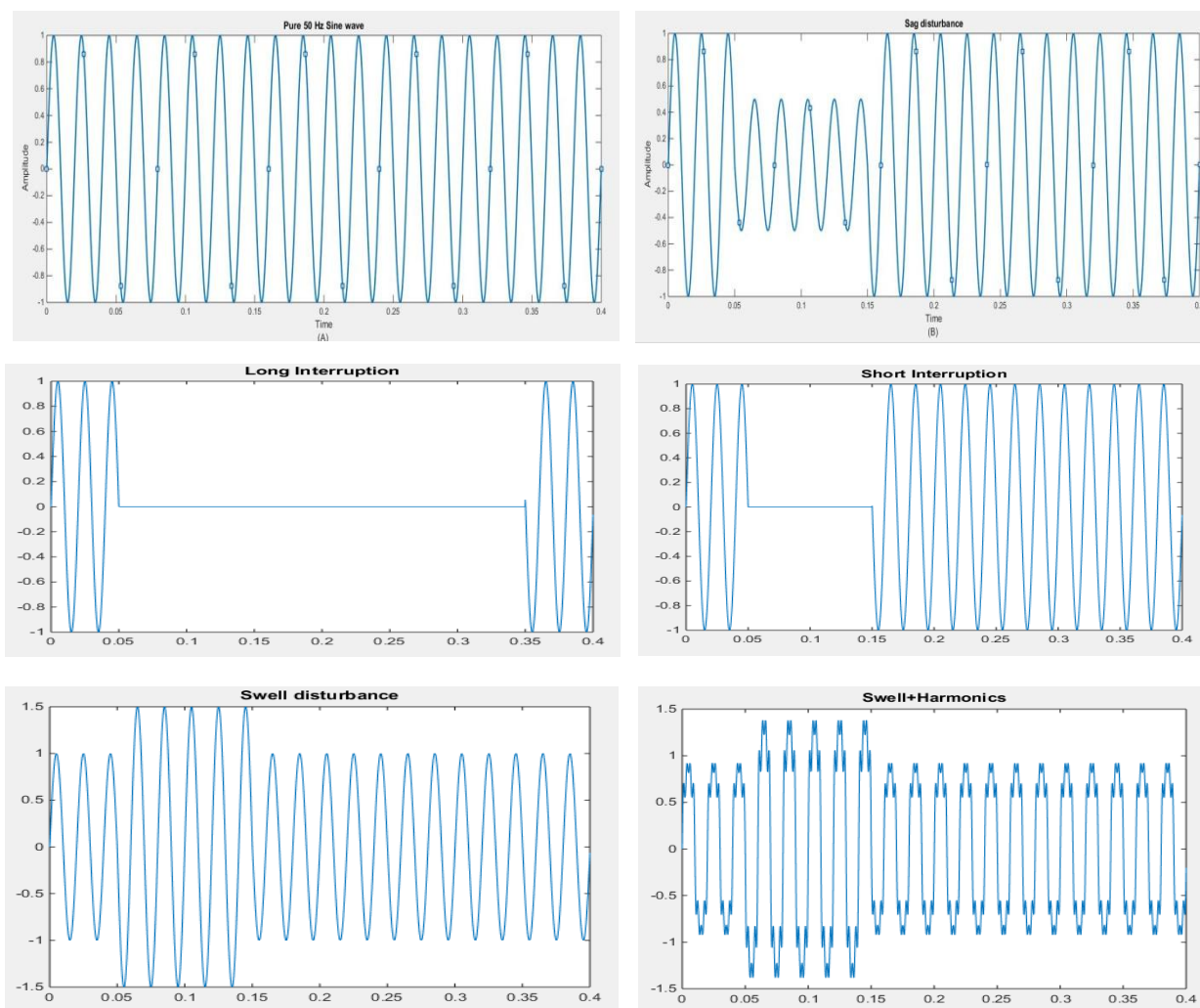
Fig 1. Power quality disturbances signal (a) Normal, (b) Pure sag, (c) long interruption, (d) short interruption, (e) swell disturbance, (f) swell with harmonics
