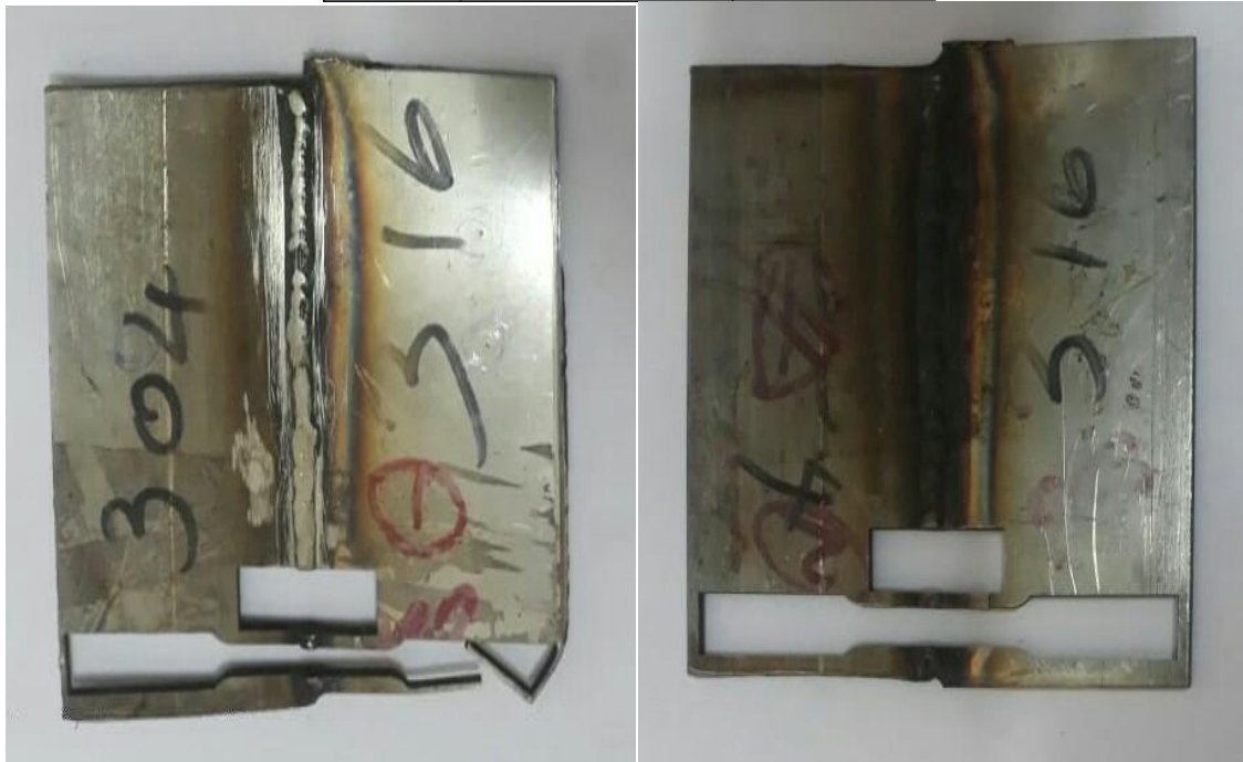
Fig. 1. Sample 1(SS304-SS316) at 100Amps Fig. 2. Sample 1(SS304-SS316) at 140Amps
