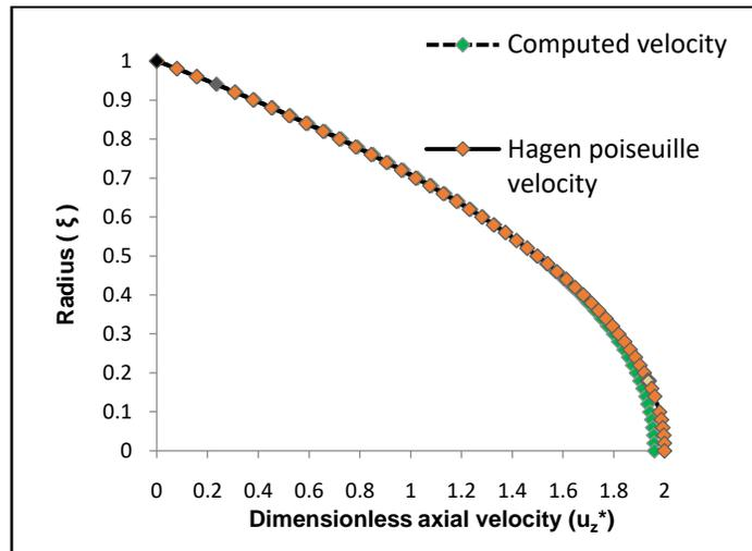
Fig.8. Comparison of axial velocity
