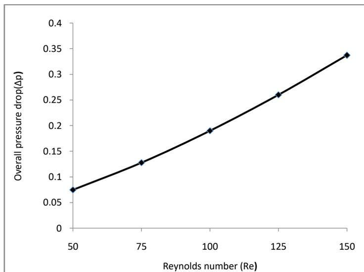
**Fig.10.** Pressure drop for various Re
