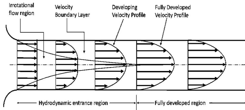
**Fig. 1.** Fully Developed flow in pipe
