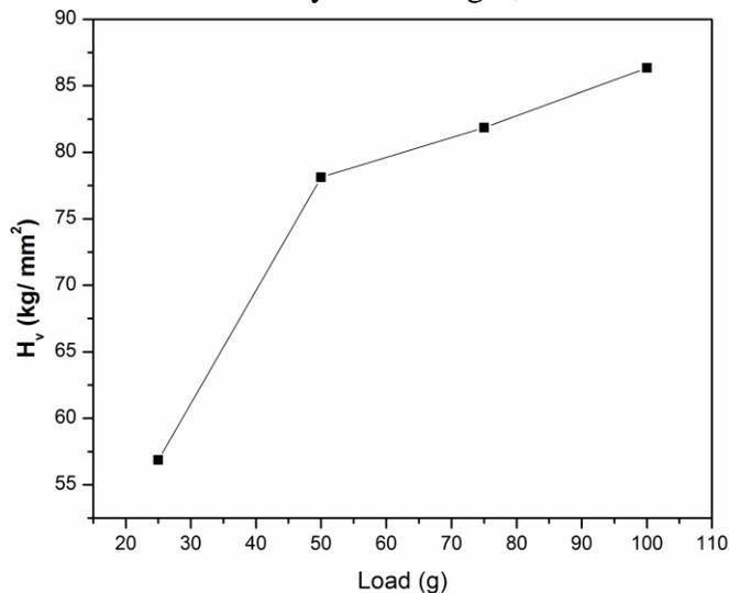
**Figure 5 Dependence of hardness number ( $H_V$ ) with loads in grams for TGSSu crystals**
