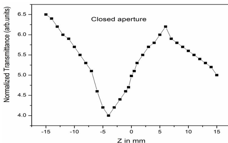
**Figure 7 Z-scan pattern for the sample in closed aperture**
