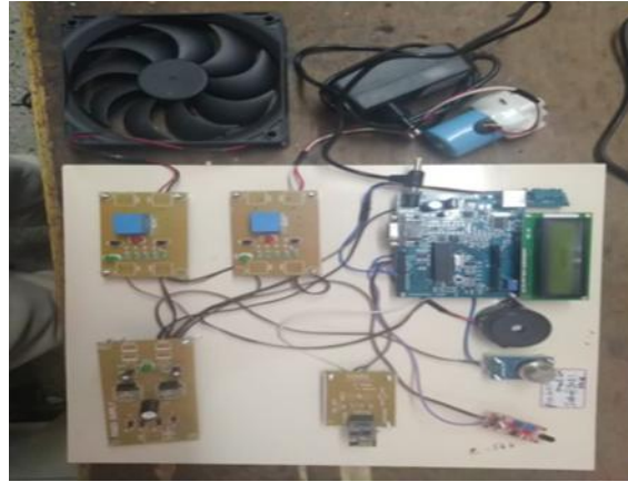
Fig4. Hardware illustration of Automatic Extinguisher.
