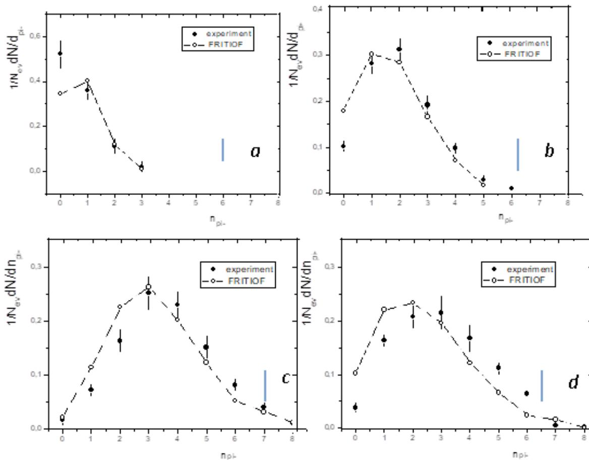
Fig.2. Multiple  $\pi$ -mesons distribution in CC interactions.a)  $n_p^{\text{par}} \leq 4$ , b)  $4 < n_p^{\text{par}} \leq 9$ , c)  $n_p^{\text{par}} > 9$ , d)  $Q_{\text{str}} = 0$ .Table 2 Relative multiplicities of  $\pi^-$  and  $\pi^+$  -mesons in CC interactions with different number of proton participants (top line – experimental results, bottom line - calculations using the FRITIOF model).
