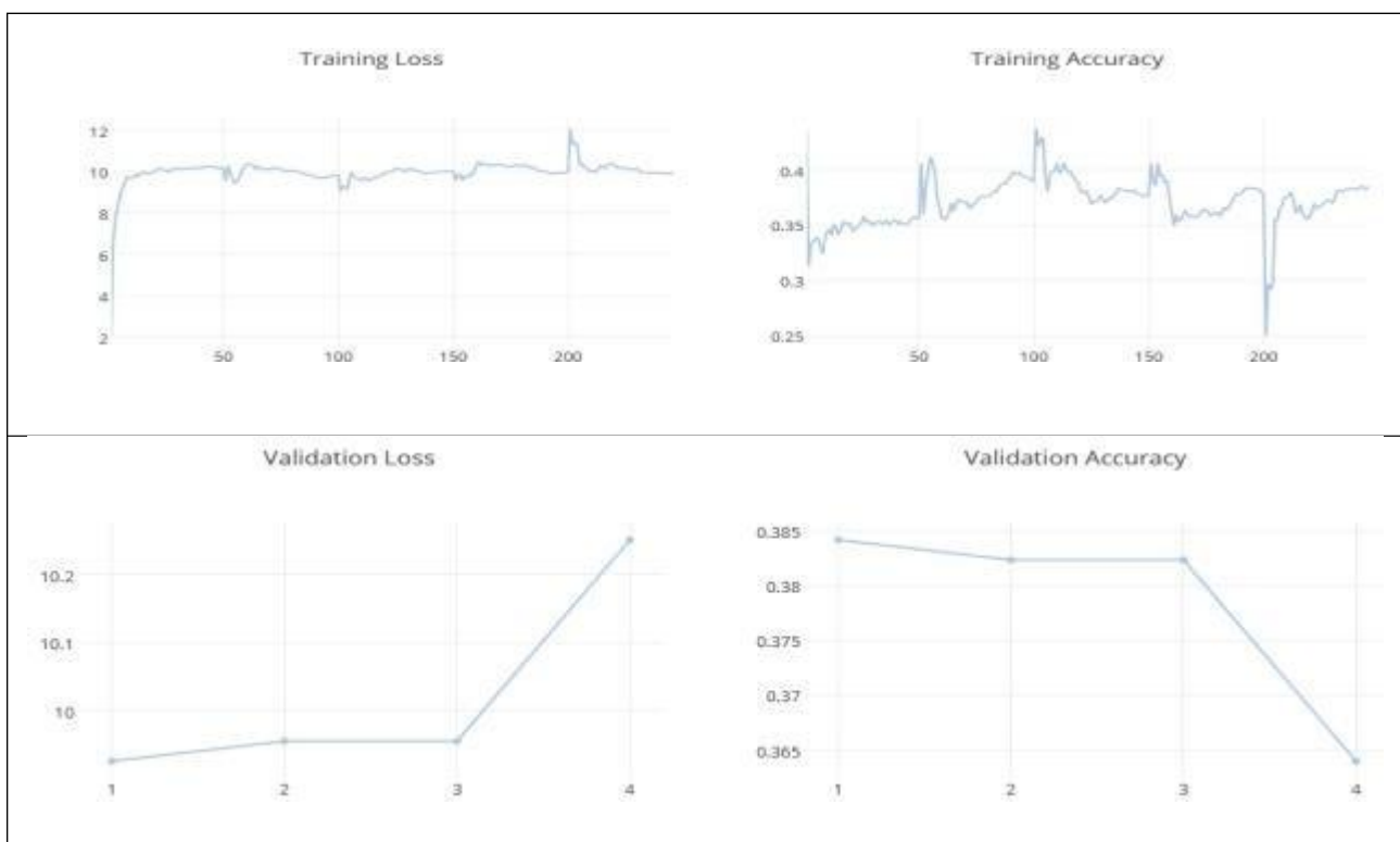
Fig.11: Plots showing training accuracy, training loss, validation accuracy and validation loss for recognizing emotions anger, stress, and neutral using InceptionV3
